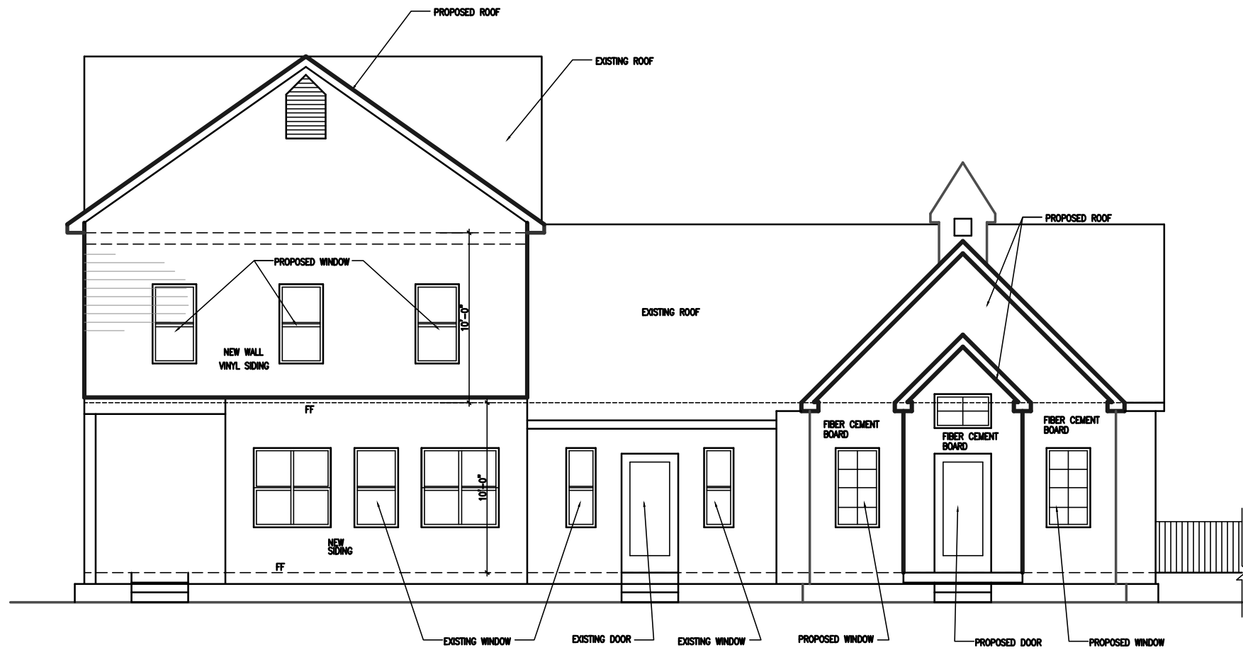
PROPOSED SOUTH-EAST ELEVATION SCALE 1/8"=1'
